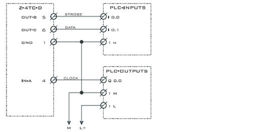
Although the connections indicated regard a SIEMENS S7-200 CPU 224-DC/DC/DC PLC in particular, other PLCs can also be used provided that their inputs are fast enough (< 2 ms) and their outputs are transistor and not relay type.
