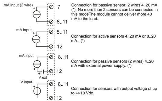
(\*) in order to utilise the input as current, the respective dip-switch must be ON. This operation connects a 100 Ohm resistance parallel to the input terminals and permits a signal of +/- 2000 mV to be obtained near +/- 20 mA.
