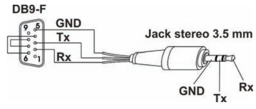
Z-PC cable creation diagram for programming by PC. This cable can be ordered as an accessory (code PM001600).
