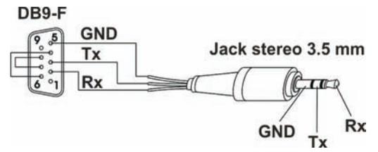
Z-PC cable creation diagram for programming by PC. This cable can be ordered as an accessory (code PM001600).
