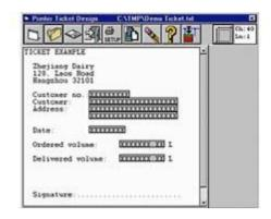
Program for design of printer tickets for the PD 4000/340 Flowmeter-Display. The program makes it possible to create a ticket layout on the PC monitor. This design is then downloaded to the PD 4000/340. A customized ticket layout may be saved on the PC hard disc for later use. Requires PD 3920/PD 3930 and VIGO software.
