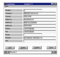
**PDFLOW** is a tool for generating a customer database for PD 4000/340 Flowmeter-Display. The database can hold up to 1200 customers. This information is then downloaded to the PD 4000/340. The PDFlow Database program is based on a standard database using Access 2.0 file format. Requires PD 3920/PD 3930 and VIGO software.
