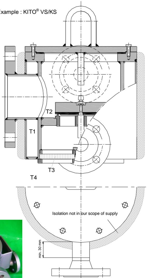
Heat loss on insulated KITO® valves or ventilation hoods.
