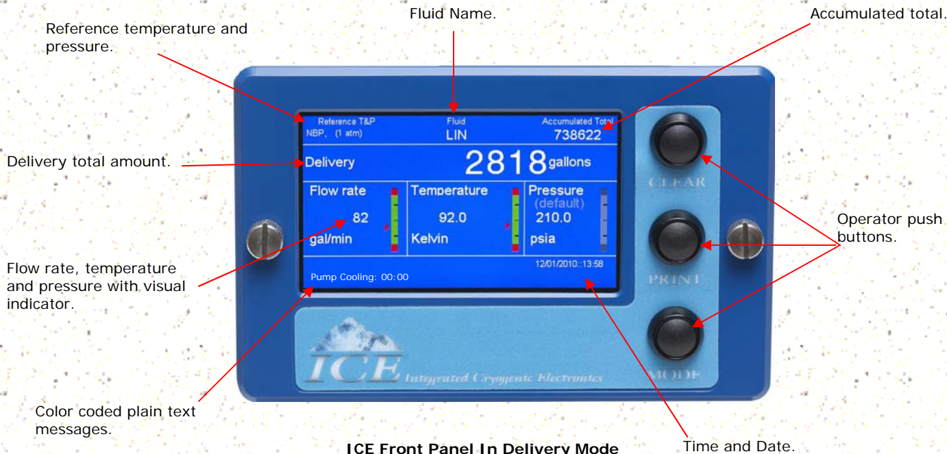
ICE Front Panel In Delivery Mode
