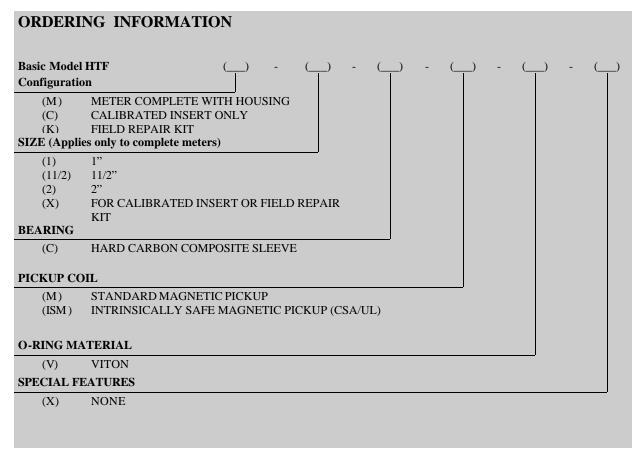
Patented design means one size internal kit fits all three meter sizes (1", 11/2" and 2").
