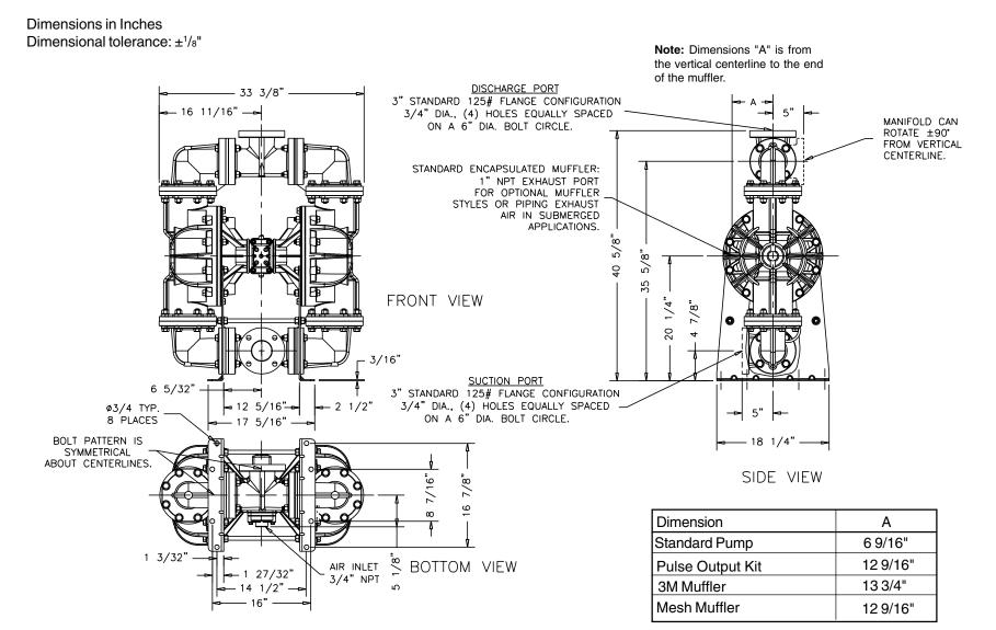
**Note:** Porting Flanges are also available with PN10 80mm DIN bolting configuration.
