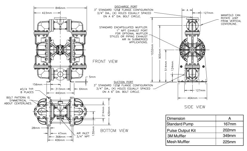
**Note:** Porting Flanges are also available with PN10 80mm DIN bolting configuration.
