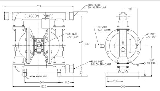
General Assembly: B40 Metallic FDA Pump, all dimensions +/- 2mm.
